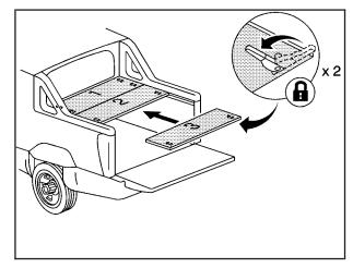
7. Push the latches away from you, starting with the left latch, to lock the panel in place. You should hear a click when each latch locks correctly.
